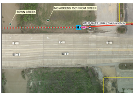
Figure 3: Redline edits collected in the GIS help ensure the accuracy of as-builts and provide useful notes
